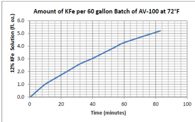
**Note:** The gel times presented in the chart above are based on controlled laboratory conditions and are for reference purpose only. It should be expected that gel times might vary on the job site. It's the sole responsibility of the user to verify and monitor gel times of their specific grout mix.
