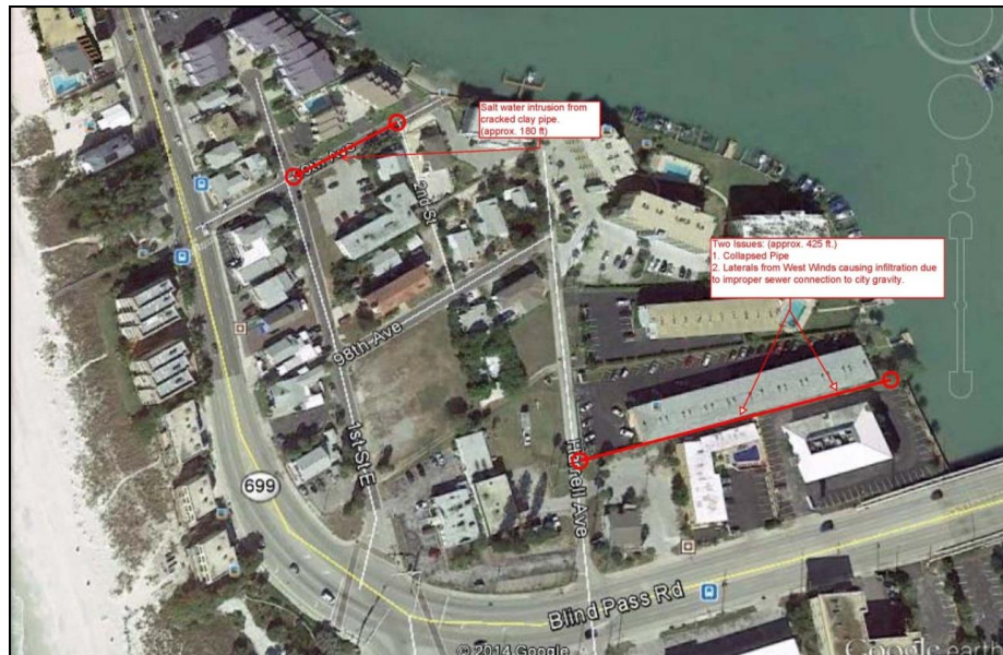
Figure 7. LS #3 Area with Extreme Infiltration
